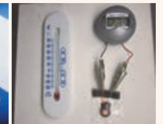
Demonstration of a solid-state battery operation at -30°C
