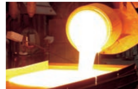
Primary melting (*1 in the right diagram)
