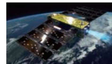
Super Low Altitude Test Satellite "TSUBAME" (SLATS) (Provided by: JAXA)
