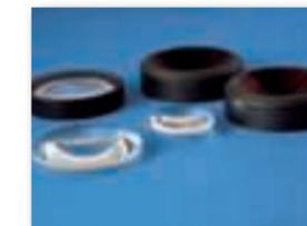
Products fabricated by heating and softening polished preforms and transferring it in an ultra-high accuracy aspheric mold and then supplied after centering and coating
