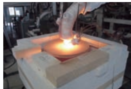
Drain casting * Pouring melted glass directly into a mold
